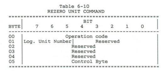
The REZERO UNIT command (Table 6-10) requests that the selected drive repositions its head(s) to cylinder zero.
