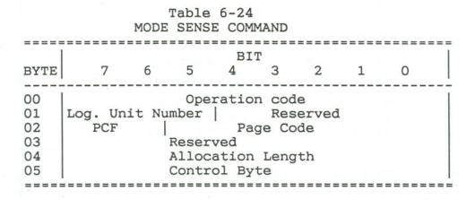
The MODE SENSE command (Table 6-24) provides a means for the target to report its peripheral device parameters to the initiator. It is a complementary command to the MODE SELECT command.
