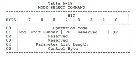
The MODE SELECT command (Table 6-19) provides a means for the initiator to specify device parameters to the controller concerning the selected LUN (drive).
