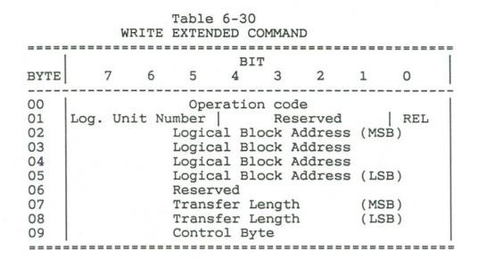
The WRITE EXTENDED command (Table 6-30) requests that the target write the data transferred by the initiator to the medium.
