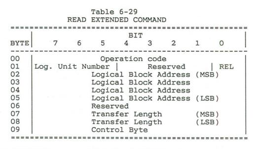
The READ EXTENDED command (Table 6-29) requests that the target transfer data to the initiator.
