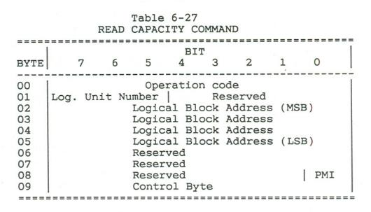
The READ CAPACITY command (Table 6-27) provides a means for the initiator to request information regarding the capacity of the disk drive.
